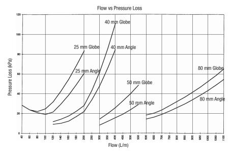
When designing a system, the industry standard maximum flow rate velocity through pipes and fittings is 2m/s. Please refer to relevant pipe velocity data.
