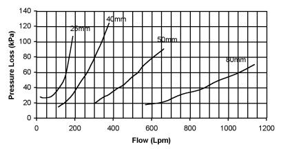
Pressure loss data are derived from valves independently tested by CIT, Fresno, CA.
