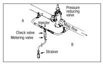
Example A. Injector installed around a point of restriction such as a regulator valve or gate valve which creates a pressure loss, thereby allowing the injector to produce a vacuum.
