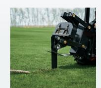
**CONSISTENT PLOWING** Optimised plow design provides down pressure to maintain consistent plowing up to 24" deep in a variety of conditions. The 10-degree frame oscillation ensures constant wheel-to-ground contact when plowing over rough terrain or crossing open trench lines.
