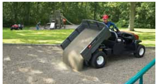
Compared to metal beds that are noisy and can rust, these double-walled polyethylene plastic beds withstand day-to-day abuse and never dent.
