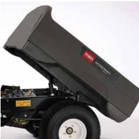
Electric Bed Lift
