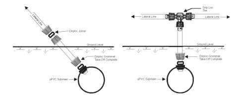
Use only slow speed hand drills. Do NOT use high speed drills. Drip-Loc® fittings can handle a range of polyethylene tubing internal diameters, as follows in the table below.
