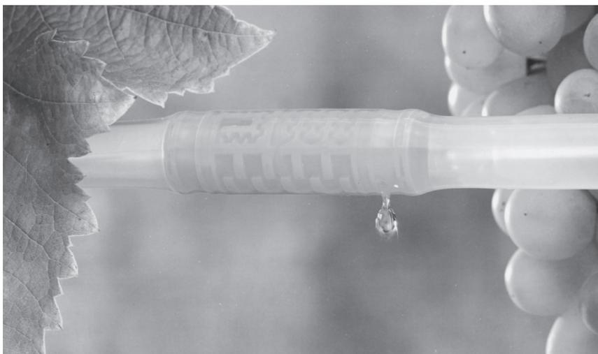
The emitter design creates turbulent flow which ensures maximum blockage resistance. The emitter is fused to the inside of the tube as it is extruded in the manufacturing process and provides substantial savings on installation costs.
