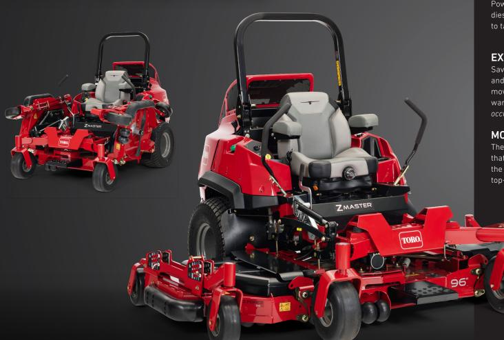
Looking for a workhorse mower that's easy to operate and gets the job done faster? Check out the Toro® Z Master® 7500-D. Highly productive 60" and 72" decks, and even a 96-inch deck design that folds up neatly for easy transport, then folds down to handle your biggest jobs — in half the time of comparable mowers.
