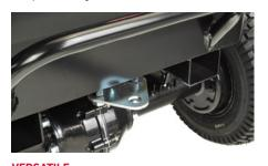
Add even more functionality, the Tow Hitch allows for optional accessories to be fitted.
