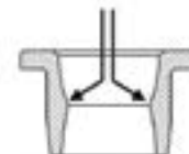
Interference barbs endure seal
