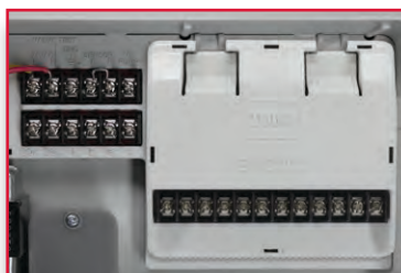
16-station configuration with (1) 12-station module
