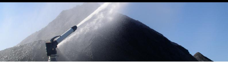
The Perrot P2M Piston Drive Sprinkler has been designed with a focus on performance. Capable of a maximum throw of up to 69 m, the P2M is an ideal solution for sports fields, agriculture and dust suppression applications.
