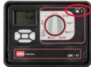
Each station can be individually set to override the rain sensor. This is useful, for example, if you have an area of your garden that is under cover and does not receive any rainfall.
