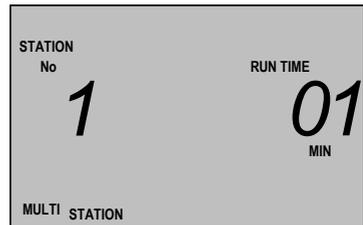
Each Station with a **Run Time** set will water in sequence, beginning with the one displayed when **P** was pressed.
