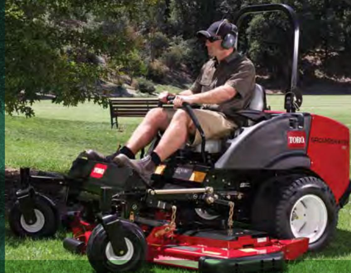
The Toro® Groundsmaster® 7200/7210 zero-radius turn rotary mowers are rugged enough to be called Groundsmasters. They have powerful Kubota® 24.8 hp (18.6 kW) or 35 hp (26 kW) 3-cylinder liquid-cooled diesel engines to get the job done. Heavy-duty 7-gauge welded steel deck construction, the industry's toughest spindle assembly, and shaft-driven cutting decks make these Groundsmasters hard to beat.
